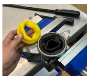
Figure 2: Push insert into voiding
