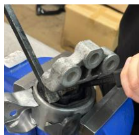
Figure 1: Secure mount in vice and pry central post out of mount
