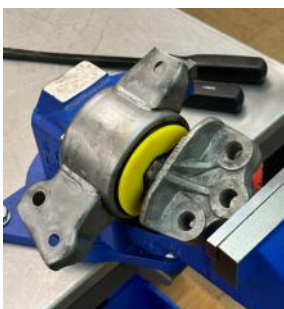
Figure 3: Push bracket/post back into place
