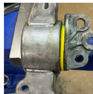
Figure 3: Push bracket/post back into place
