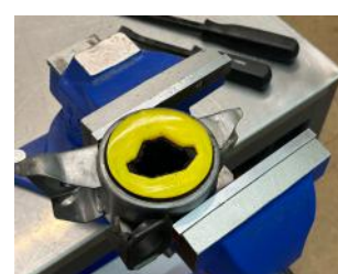
Figure 1: Secure mount in vice and pry central post out of mount
