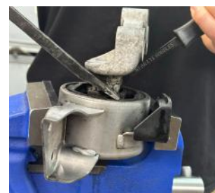
Figure 1: Secure mount in vice and pry central post out of mount
