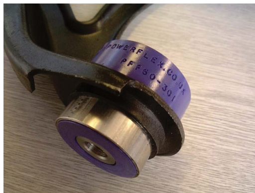
Figure 1- Bush fitted in wishbone
